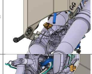
Upper mounting brackets install as shown at right with 6mm spacers and M8 x 40 bolts. Torque bolts per factory specification of 19 Nm.
